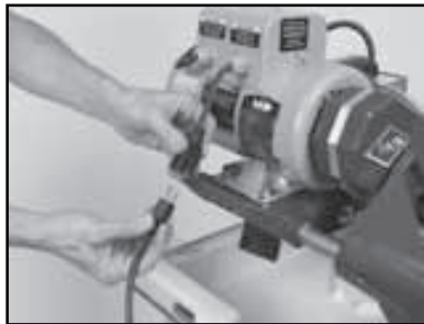
(B) Connect the Water Pump power cord to the connection found on the back of the motor.
