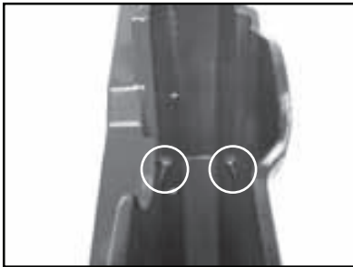
(D) Verify proper cooling flow on both sides of the blade (See Maintenance Section to increase/decrease flow).
