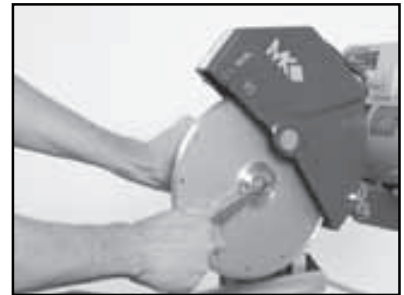
(F) Install Retaining Nut and Outer Flange, depress and hold the Shaft Lock pushbutton and tighten Retaining Nut.
