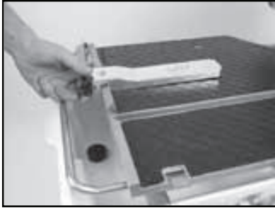
(A) Remove the Adjustable Cutting Guide.
