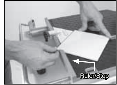
(C) Place tile on the Cutting Table.
