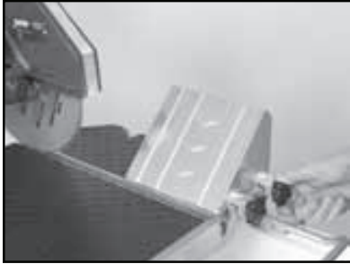
(A) Position the 45° Bullnose Miter Guide and tighten the retaining thumbscrew.
