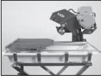
(A) Position Movable Cutting Table to the front of the saw and raise the Blade Guard by loosening the wingnut.
