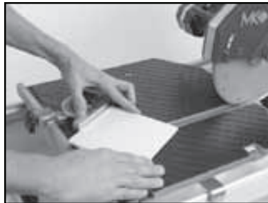
(D) Position the tile against the 90° Protractor and the Ruler/Stop. Turn the motor ON.
