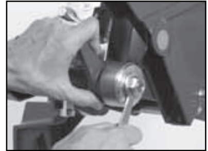
(C) Depress and hold the Shaft Lock pushbutton and remove Retaining Nut and Outer Flange using the Blade Wrench.
