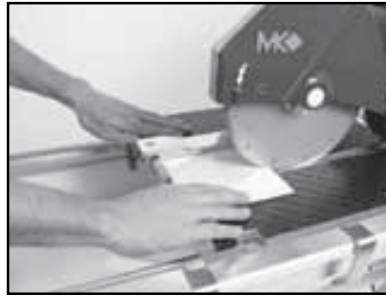
(E) Perform the cut. Turn the motor OFF when work is complete.
