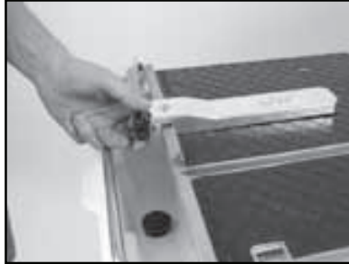
(B) Tighten the retaining thumbscrew.
