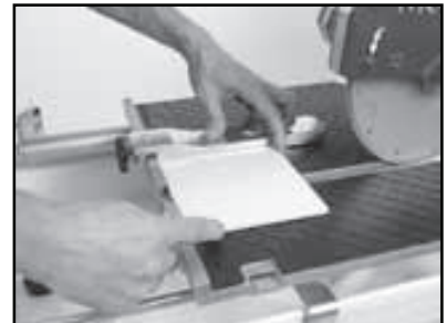
(C) Place the tile against the Ruler/Stop and Cutting Guide. Turn the motor ON.
