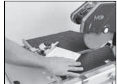
(F) Perform the cut. Turn the motor OFF when work is complete.
