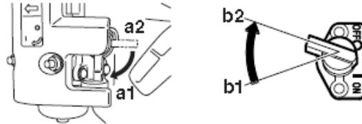
1. Open Fuel Valve by moving lever down (a1).
